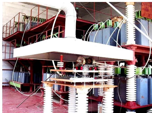
Fig. 1. General view of a powerful high-voltage high-current generator of artificial lightning current of the type YITOM-1 (in the foreground there is a desktop with a high-voltage three-electrode air controlled switch with steel electrodes for a voltage of \pm 50 kV and pulsed sinusoidal lightning current up to \pm 220 kA, a tested sample of the skin of an aircraft and an air drawing system, and in the background – separate high-voltage pulse current generators for the corresponding current components A , B , C , C^* and D ) [11]
