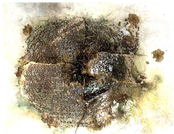
Fig. 6. The results of the action of an artificial lightning current pulse ( I_{mA} \approx -212 \text{ kA} ) on a prototype aircraft skin made of multilayer CM using fiberglass, carbon fiber, and metal mesh [18]
