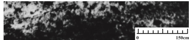
Fig. 5. Microsection of the polished surface. Dark tempering field and white austenite spots. \times 150
